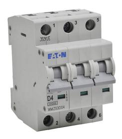
Eaton miniature supplementary protector, 4A, 480Y/277 VAC/96 VDC, 3-pole, D curve, thermal magnetic, 35mm DIN rail mount.
