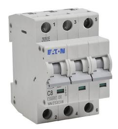
Eaton miniature supplementary protector, 8A, 480Y/277 VAC/96 VDC, 3-pole, C curve, thermal magnetic, 35mm DIN rail mount.
