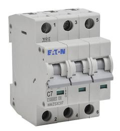
Eaton miniature supplementary protector, 7A, 480Y/277 VAC/96 VDC, 3-pole, C curve, thermal magnetic, 35mm DIN rail mount.
