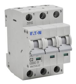
Eaton miniature supplementary protector, 2A, 480Y/277 VAC/96 VDC, 3-pole, C curve, thermal magnetic, 35mm DIN rail mount.
