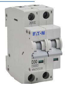
Eaton miniature supplementary protector, 30A, 480Y/277 VAC/96 VDC, 2-pole, D curve, thermal magnetic, 35mm DIN rail mount.
