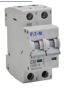
Eaton miniature supplementary protector, 32A, 480Y/277 VAC/96 VDC, 2-pole, C curve, thermal magnetic, 35mm DIN rail mount.
