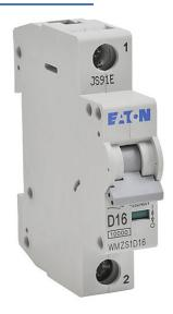
Eaton miniature supplementary protector, 16A, 277 VAC/48 VDC, 1-pole, D curve, thermal magnetic, 35mm DIN rail mount.
