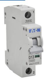
Eaton miniature supplementary protector, 13A, 277 VAC/48 VDC, 1-pole, D curve, thermal magnetic, 35mm DIN rail mount.
