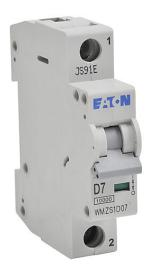
Eaton miniature supplementary protector, 7A, 277 VAC/48 VDC, 1-pole, D curve, thermal magnetic, 35mm DIN rail mount.
