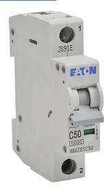
Eaton miniature supplementary protector, 50A, 277 VAC/48 VDC, 1-pole, C curve, thermal magnetic, 35mm DIN rail mount.
