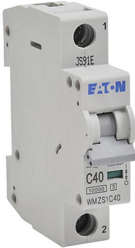
Eaton miniature supplementary protector, 40A, 277 VAC/48 VDC, 1-pole, C curve, thermal magnetic, 35mm DIN rail mount.
