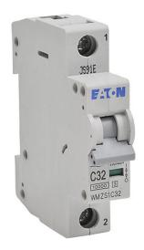
Eaton miniature supplementary protector, 32A, 277 VAC/48 VDC, 1-pole, C curve, thermal magnetic, 35mm DIN rail mount.
