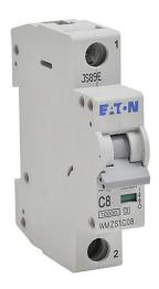
Eaton miniature supplementary protector, 8A, 277 VAC/48 VDC, 1-pole, C curve, thermal magnetic, 35mm DIN rail mount.
