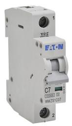
Eaton miniature supplementary protector, 7A, 277 VAC/48 VDC, 1-pole, C curve, thermal magnetic, 35mm DIN rail mount.
