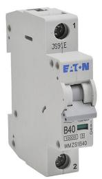
Eaton miniature supplementary protector, 40A, 277 VAC/48 VDC, 1-pole, B curve, thermal magnetic, 35mm DIN rail mount.
