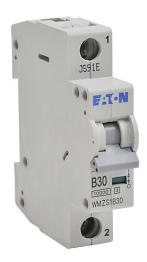
Eaton miniature supplementary protector, 30A, 277 VAC/48 VDC, 1-pole, B curve, thermal magnetic, 35mm DIN rail mount.
