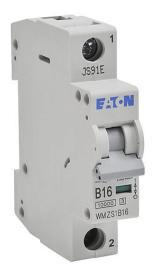
Eaton miniature supplementary protector, 16A, 277 VAC/48 VDC, 1-pole, B curve, thermal magnetic, 35mm DIN rail mount.
