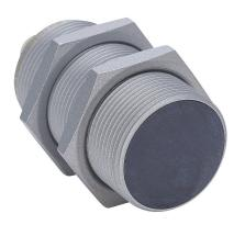
AutomationDirect inductive proximity sensor, tubular, 30mm diameter x 65mm body, weld coated brass housing, PNP, N.O. output, 15mm sensing distance, flush, 2 kHz switching frequency, IP65 IP66 IP67 IP68 IP69K, 4-pin M12 quick-disconnect.
