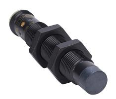
AutomationDirect inductive proximity sensor, tubular, 12mm diameter x 65mm body, weld coated brass housing, PNP, N.O. output, 8mm sensing distance, non-flush, 2 kHz switching frequency, IP67, 4-pin M12 quick-disconnect.
