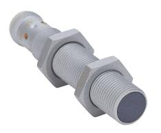
AutomationDirect inductive proximity sensor, tubular, 12mm diameter x 65mm body, weld coated brass housing, PNP, N.O. output, 4mm sensing distance, flush, 2 kHz switching frequency, IP65 IP66 IP67 IP68 IP69K, 4-pin M12 quick-disconnect.
