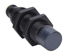
AutomationDirect inductive proximity sensor, tubular, 18mm diameter x 65mm body, weld coated brass housing, PNP, N.O. output, 12mm sensing distance, non-flush, 2 kHz switching frequency, IP67, 4-pin M12 quick-disconnect.
