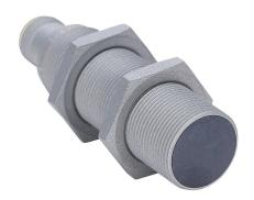
AutomationDirect inductive proximity sensor, tubular, 18mm diameter x 65mm body, weld coated brass housing, PNP, N.O. output, 8mm sensing distance, flush, 2 kHz switching frequency, IP65 IP66 IP67 IP68 IP69K, 4-pin M12 quick-disconnect.
