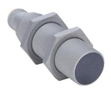
AutomationDirect inductive proximity sensor, tubular, 18mm diameter x 65mm body, weld coated brass housing, PNP, N.O. output, 8mm sensing distance, flush, 2 kHz switching frequency, IP65 IP66 IP67 IP68 IP69K, 4-pin M12 quick-disconnect.
