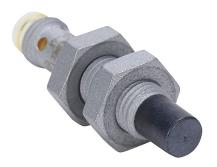
AutomationDirect inductive proximity sensor, tubular, 8mm diameter x 40mm body, weld coated 316 stainless steel housing, PNP, N.O. output, 6mm sensing distance, non-flush, 2 kHz switching frequency, IP65 IP66 IP67 IP68 IP69K, 3-pin M8 quickdisconnect.
