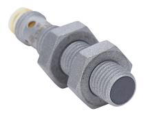
AutomationDirect inductive proximity sensor, tubular, 8mm diameter x 40mm body, weld coated 316 stainless steel housing, PNP, N.O. output, 3mm sensing distance, flush, 2 kHz switching frequency, IP65 IP66 IP67 IP68 IP69K, 3-pin M8 quick-disconnect.
