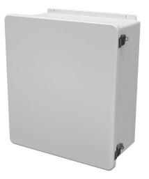
Stahlin J series enclosure, NEMA 1/3R/4X/6P/12, 18 x 16 x 8in (HxWxD), wall mount, fiberglass reinforced polyester, white, single-door, (2) quick-release latches, padlock hasp and staple.
