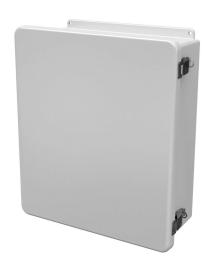
Stahlin J series enclosure, NEMA 1/3R/4X/6P/12, 16 x 14 x 6in (HxWxD), wall mount, fiberglass reinforced polyester, white, single-door, (2) quick-release latches, padlock hasp and staple.
