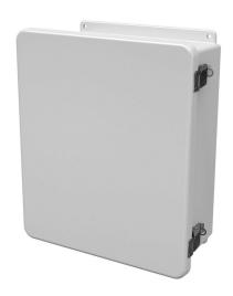
Stahlin J series enclosure, NEMA 1/3R/4X/6P/12, 14 x 12 x 6in (HxWxD), wall mount, fiberglass reinforced polyester, white, single-door, (2) quick-release latches, padlock hasp and staple.
