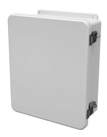
Stahlin J series enclosure, NEMA 1/3R/4X/6P/12, 12 x 10 x 5in (HxWxD), wall mount, fiberglass reinforced polyester, white, single-door, (2) quick-release latches, padlock hasp and staple.
