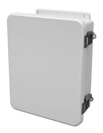
Stahlin J series enclosure, NEMA 1/3R/4X/6P/12, 10 x 8 x 4in (HxWxD), wall mount, fiberglass reinforced polyester, white, single-door, (2) quick-release latches, padlock hasp and staple.
