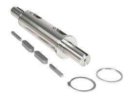
IronHorse gearbox double output shaft, 1.25in. For use with WGSS-262 series gearboxes. (4) keys, (1) retaining ring and (1) C-clip included.
