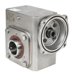
IronHorse heavy duty worm gearbox, 60:1 ratio, 56C-Face input, hollow, 1.9375in diameter output shaft, nominal 0.89hp at 1.0 SF, 1279 lb-in mechanical output torque, 2-5/8in center distance, 304 stainless steel housing, top and bottom mount.
