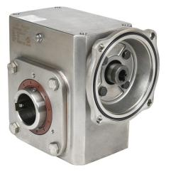
IronHorse heavy duty worm gearbox, 50:1 ratio, 56C-Face input, hollow, 1.9375in diameter output shaft, nominal 1.08hp at 1.0 SF, 1423 lb-in mechanical output torque, 2-5/8in center distance, 304 stainless steel housing, top and bottom mount.
