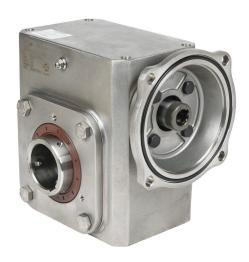
IronHorse heavy duty worm gearbox, 40:1 ratio, 56C-Face input, hollow, 1.9375in diameter output shaft, nominal 1.33hp at 1.0 SF, 1454 lb-in mechanical output torque, 2-5/8in center distance, 304 stainless steel housing, top and bottom mount.
