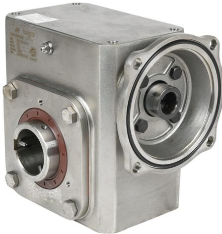
IronHorse heavy duty worm gearbox, 30:1 ratio, 145TC-Face input, hollow, 1.9375in diameter output shaft, nominal 1.68hp at 1.0 SF, 1446 lb-in mechanical output torque, 2-5/8in center distance, 304 stainless steel housing, top and bottom mount.
