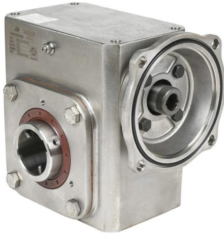
IronHorse heavy duty worm gearbox, 30:1 ratio, 56C-Face input, hollow, 1.9375in diameter output shaft, nominal 1.68hp at 1.0 SF, 1446 lb-in mechanical output torque, 2-5/8in center distance, 304 stainless steel housing, top and bottom mount.
