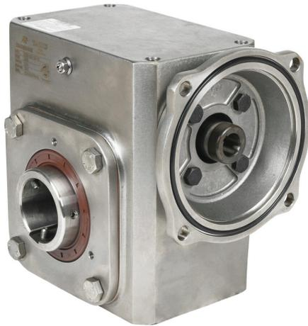
IronHorse heavy duty worm gearbox, 20:1 ratio, 56C-Face input, hollow, 1.9375in diameter output shaft, nominal 2.36hp at 1.0 SF, 1472 lb-in mechanical output torque, 2-5/8in center distance, 304 stainless steel housing, top and bottom mount.
