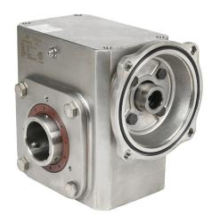
IronHorse heavy duty worm gearbox, 15:1 ratio, 145TC-Face input, hollow, 1.9375in diameter output shaft, nominal 2.96hp at 1.0 SF, 1415 lb-in mechanical output torque, 2-5/8in center distance, 304 stainless steel housing, top and bottom mount.
