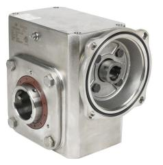
IronHorse heavy duty worm gearbox, 10:1 ratio, 145TC-Face input, hollow, 1.9375in diameter output shaft, nominal 3.96hp at 1.0 SF, 1301 lb-in mechanical output torque, 2-5/8in center distance, 304 stainless steel housing, top and bottom mount.
