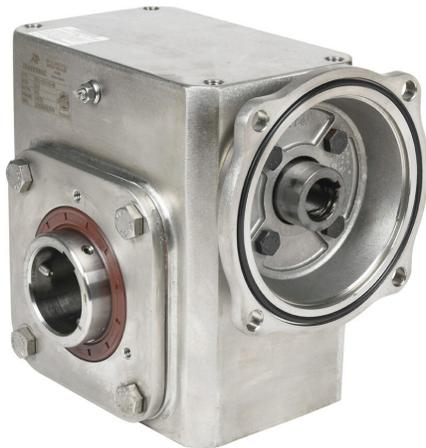
IronHorse heavy duty worm gearbox, 10:1 ratio, 145TC-Face input, hollow, 1.9375in diameter output shaft, nominal 3.96hp at 1.0 SF, 1301 lb-in mechanical output torque, 2-5/8in center distance, 304 stainless steel housing, top and bottom mount.
