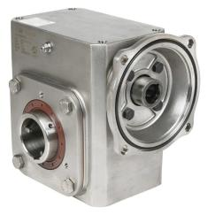
IronHorse heavy duty worm gearbox, 5:1 ratio, 145TC-Face input, hollow, 1.9375in diameter output shaft, nominal 5.24hp at 1.0 SF, 933 lb-in mechanical output torque, 2-5/8in center distance, 304 stainless steel housing, top and bottom mount.
