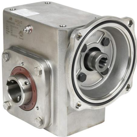
IronHorse heavy duty worm gearbox, 60:1 ratio, 56C-Face input, hollow, 1.4375in diameter output shaft, nominal 0.71hp at 1.0 SF, 1008 lb-in mechanical output torque, 2-3/8in center distance, 304 stainless steel housing, top and bottom mount.
