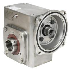
IronHorse heavy duty worm gearbox, 60:1 ratio, 56C-Face input, hollow, 1.4375in diameter output shaft, nominal 0.71hp at 1.0 SF, 1008 lb-in mechanical output torque, 2-3/8in center distance, 304 stainless steel housing, top and bottom mount.
