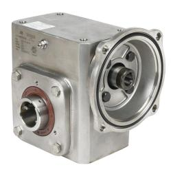
IronHorse heavy duty worm gearbox, 50:1 ratio, 56C-Face input, hollow, 1.4375in diameter output shaft, nominal 0.87hp at 1.0 SF, 1111 lb-in mechanical output torque, 2-3/8in center distance, 304 stainless steel housing, top and bottom mount.
