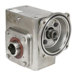
IronHorse heavy duty worm gearbox, 30:1 ratio, 56C-Face input, hollow, 1.4375in diameter output shaft, nominal 1.33hp at 1.0 SF, 1105 lb-in mechanical output torque, 2-3/8in center distance, 304 stainless steel housing, top and bottom mount.
