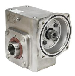
IronHorse heavy duty worm gearbox, 20:1 ratio, 56C-Face input, hollow, 1.4375in diameter output shaft, nominal 2.01hp at 1.0 SF, 1243 lb-in mechanical output torque, 2-3/8in center distance, 304 stainless steel housing, top and bottom mount.
