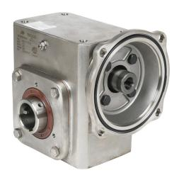
IronHorse heavy duty worm gearbox, 15:1 ratio, 56C-Face input, hollow, 1.4375in diameter output shaft, nominal 2.36hp at 1.0 SF, 1108 lb-in mechanical output torque, 2-3/8in center distance, 304 stainless steel housing, top and bottom mount.
