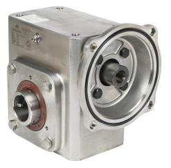
IronHorse heavy duty worm gearbox, 10:1 ratio, 56C-Face input, hollow, 1.4375in diameter output shaft, nominal 3.23hp at 1.0 SF, 1055 lb-in mechanical output torque, 2-3/8in center distance, 304 stainless steel housing, top and bottom mount.
