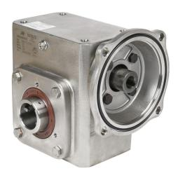
IronHorse heavy duty worm gearbox, 5:1 ratio, 56C-Face input, hollow, 1.4375in diameter output shaft, nominal 4.32hp at 1.0 SF, 767 lb-in mechanical output torque, 2-3/8in center distance, 304 stainless steel housing, top and bottom mount.
