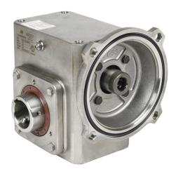
IronHorse heavy duty worm gearbox, 60:1 ratio, 56C-Face input, hollow, 1.4375in diameter output shaft, nominal 0.52hp at 1.0 SF, 777 lb-in mechanical output torque, 2-1/16in center distance, 304 stainless steel housing, top and bottom mount.
