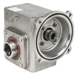
IronHorse heavy duty worm gearbox, 50:1 ratio, 56C-Face input, hollow, 1.4375in diameter output shaft, nominal 0.6hp at 1.0 SF, 771 lb-in mechanical output torque, 2-1/16in center distance, 304 stainless steel housing, top and bottom mount.
