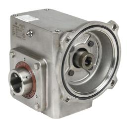
IronHorse heavy duty worm gearbox, 40:1 ratio, 56C-Face input, hollow, 1.4375in diameter output shaft, nominal 0.76hp at 1.0 SF, 774 lb-in mechanical output torque, 2-1/16in center distance, 304 stainless steel housing, top and bottom mount.
