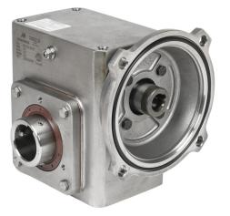
IronHorse heavy duty worm gearbox, 30:1 ratio, 56C-Face input, hollow, 1.4375in diameter output shaft, nominal 0.95hp at 1.0 SF, 802 Ib-in mechanical output torque, 2-1/16in center distance, 304 stainless steel housing, top and bottom mount.
